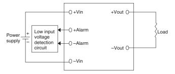
The input voltage detection output terminal (±Alarm) is a transistor output of a photo-coupler and it is insulated at the both input and output sides.
