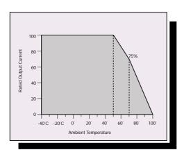
Derating Curve Output Current vs Temperature S3V3 Natural Convection (<0.1m/s airflow)
