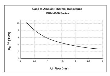
For design margin and to enhance system reliability, it is recommended that the PKM 4000 series DC/DC power modules are operated at case temperatures below  $90^{\circ}\text{C}.$
