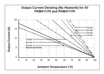
The graphs below can be used to estimate case temperatures for given system operating conditions (see Thermal Design). For further information on optional heatsinks, please contact your local Ericsson sales office.
